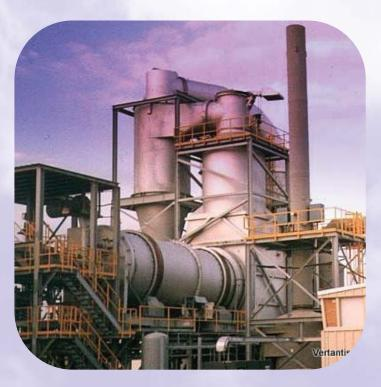
The Rotary Kiln comprises a rotating drum for combustion of waste solids, slurries and sludges and a secondary combustion chamber for complete destruction of the wastes
