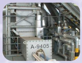
"Hydraulic Ram" may be supplied for direct input of waste solids. Depending on density, slurries and sludges may be introduced into the Ram or atomized through a burner. Rotating drum can be adjusted to provide sufficient residence time to "burn" the wastes
