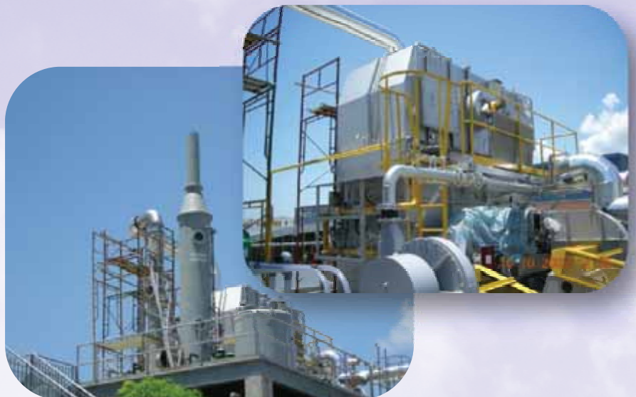
Thermal Oxidizer treating VOC comprising organics and chlorinated wastes at flexible printed circuit manufacturer in Singapore. System includes HCl treatment.
